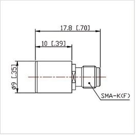
RF Solution offer a wide selection of Coaxial Fixed Termination (Dummy Load) for global customers. CT-02W-RA0910-SK-18G is a Coaxial Fixed Termination (Dummy Load) in Frequency Range of DC~18.0 GHz. It is made of high quality materials under a high standard, the Connector Type of this product is SMA-F (K), VSWR Max is 1.30 and Impedance is 50  $\Omega$ . The component has a good working performance and stability, it is ideal for handling a Power of 2 W.
