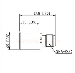
RF Solution offer a wide selection of Coaxial Fixed Termination (Dummy Load) for global customers. CT-02W-RA0910-SK-10G is a Coaxial Fixed Termination (Dummy Load) in Frequency Range of DC~10.0 GHz. It is made of high quality materials under a high standard, the Connector Type of this product is SMA-F (K), VSWR Max is 1.25 and Impedance is 50  $\Omega$ . The component has a good working performance and stability, it is ideal for handling a Power of 2 W.
