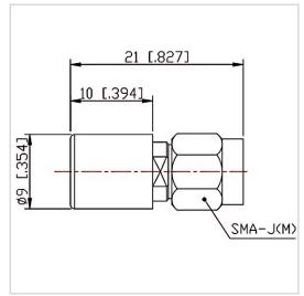
RF Solution offer a wide selection of Coaxial Fixed<br/>Termination (Dummy Load) for global customers.<br/>CT-02W-RA0910-SJ-8G is a Coaxial Fixed Termination<br/>(Dummy Load) in Frequency Range of DC~8.0 GHz. It<br/>is made of high quality materials under a high<br/>standard, the Connector Type of this product is SMA-<br/>M (J), VSWR Max is 1.20 and Impedance is 50 Ω. The<br/>component has a good working performance and<br/>stability, it is ideal for handling a Power of 2 W.
