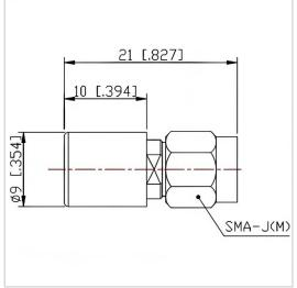
RF Solution offer a wide selection of Coaxial Fixed Termination (Dummy Load) for global customers. CT-02W-RA0910-SJ-6G is a Coaxial Fixed Termination (Dummy Load) in Frequency Range of DC $\sim$ 6.0 GHz. It is made of high quality materials under a high standard, the Connector Type of this product is SMA-M (J), VSWR Max is 1.20 and Impedance is 50  $\Omega$ . The component has a good working performance and stability, it is ideal for handling a Power of 2 W.
