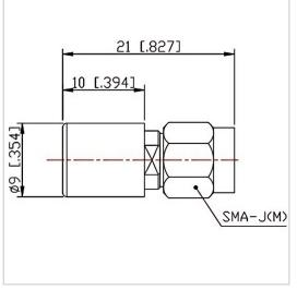
RF Solution offer a wide selection of Coaxial Fixed Termination (Dummy Load) for global customers. CT-02W-RA0910-SJ-18G is Coaxial Fixed а Termination (Dummy Load) in Frequency Range of DC~18.0 GHz. It is made of high quality materials under a high standard, the Connector Type of this product is SMA-M (J), VSWR Max is 1.30 and SMA-J(M) Impedance is 50  $\Omega$ . The component has a good working performance and stability, it is ideal for handling a Power of 2 W.
