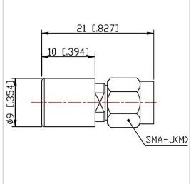
RF Solution offer a wide selection of Coaxial Fixed Termination (Dummy Load) for global customers. CT-02W-RA0910-SJ-10G is a Coaxial Fixed Termination (Dummy Load) in Frequency Range of DC~10.0 GHz. It is made of high quality materials under a high standard, the Connector Type of this product is SMA-M (J), VSWR Max is 1.25 and Impedance is 50  $\Omega$ . The component has a good working performance and stability, it is ideal for handling a Power of 2 W.
