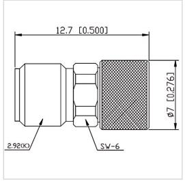
RF Solution offer a wide selection of Coaxial Fixed Termination (Dummy Load) for global customers. CT-02W-RA0713-2.92K-40G is a Coaxial Termination (Dummy Load) in Frequency Range of DC~40.0 GHz. It is made of high quality materials under a high standard, the Connector Type of this product is 2.92-F (K), VSWR Max is 1.20 and Impedance is 50  $\Omega$ . The component has a good working performance and stability, it is ideal for handling a Power of 2 W.
