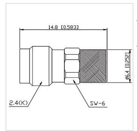
RF Solution offer a wide selection of Coaxial Fixed Termination (Dummy Load) for global customers. CT-02W-RA0615-2.4K-50G is a Coaxial Fixed Termination (Dummy Load) in Frequency Range of DC~50.0 GHz. It is made of high quality materials under a high standard, the Connector Type of this product is 2.4-F (K), VSWR Max is 1.20 and Impedance is 50  $\Omega$ . The component has a good working performance and stability, it is ideal for handling a Power of 2 W.
