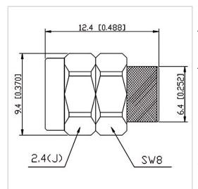
RF Solution offer a wide selection of Coaxial Fixed Termination (Dummy Load) for global customers. CT-02W-RA0612-2.4J-50G is a Coaxial Fixed Termination (Dummy Load) in Frequency Range of DC~50.0 GHz. It is made of high quality materials under a high standard, the Connector Type of this product is 2.4-M (J), VSWR Max is 1.20 and Impedance is 50  $\Omega$ . The component has a good working performance and stability, it is ideal for handling a Power of 2 W.
