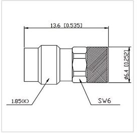
RF Solution offer a wide selection of Coaxial Fixed Termination (Dummy Load) for global customers. CT-02W-RA0612-1.85K-67G is a Coaxial Termination (Dummy Load) in Frequency Range of DC~67.0 GHz. It is made of high quality materials under a high standard, the Connector Type of this product is 1.85-F (K), VSWR Max is 1.30 and Impedance is 50  $\Omega$ . The component has a good working performance and stability, it is ideal for handling a Power of 2 W.
