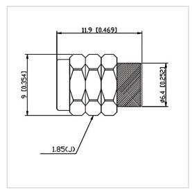
RF Solution offer a wide selection of Coaxial Fixed Termination (Dummy Load) for global customers. CT-02W-RA0612-1.85J-67G is a Coaxial Termination (Dummy Load) in Frequency Range of DC~67.0 GHz. It is made of high quality materials under a high standard, the Connector Type of this product is 1.85-M (J), VSWR Max is 1.30 and Impedance is 50  $\Omega$ . The component has a good working performance and stability, it is ideal for handling a Power of 2 W.
