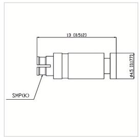
RF Solution offer a wide selection of Coaxial Fixed Termination (Dummy Load) for global customers. CT-02W-RA0515-SMPK-40G is a Coaxial Fixed Termination (Dummy Load) in Frequency Range of DC~40.0 GHz. It is made of high quality materials under a high standard, the Connector Type of this product is SMP-F (K), VSWR Max is 1.30 and Impedance is 50  $\Omega$ . The component has a good working performance and stability, it is ideal for handling a Power of 2 W.
