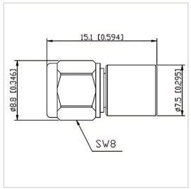
RF Solution offer a wide selection of Coaxial Fixed Termination (Dummy Load) for global customers. CT-01W-RA0815-1.35J-90G is a Coaxial Fixed Termination (Dummy Load) in Frequency Range of DC~90.0 GHz. It is made of high quality materials under a high standard, the Connector Type of this product is 1.35-F (K), VSWR Max is 1.60 and Impedance is 50  $\Omega$ . The component has a good working performance and stability, it is ideal for handling a Power of 1 W.
