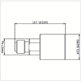
RF Solution offer a wide selection of Coaxial Fixed Termination (Dummy Load) for global customers. CT-01W-RA0814-1.0K-110G is a Coaxial Fixed Termination (Dummy Load) in Frequency Range of DC~110.0 GHz. It is made of high quality materials under a high standard, the Connector Type of this product is 1.0-F (K), VSWR Max is 1.50 and Impedance is 50  $\Omega$ . The component has a good working performance and stability, it is ideal for handling a Power of 1 W.
