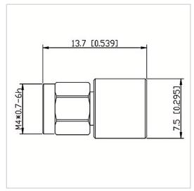
RF Solution offer a wide selection of Coaxial Fixed Termination (Dummy Load) for global customers. CT-01W-RA0814-1.0J-110G is a Coaxial Fixed Termination (Dummy Load) in Frequency Range of DC~110.0 GHz. It is made of high quality materials under a high standard, the Connector Type of this product is 1.0-M (J), VSWR Max is 1.50 and Impedance is 50  $\Omega$ . The component has a good working performance and stability, it is ideal for handling a Power of 1 W.
