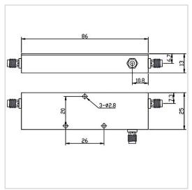
RF Solution offer a wide selection of Coupler for global customers. CP20-F2586-S-0.698-2.2GHz is a Coupler in Frequency Range of  $0.698\sim2.2$  GHz. It is made of high quality materials under a high standard, the Insertion Loss Max of this product is 0.4 dB, Nominal Coupling is  $20\pm1$  dB and Coupling Sensitivity is  $\pm$  0.6 dB. The component has a good working performance and stability, it is ideal for handling a Rated Power of 50 W.
