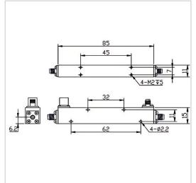
RF Solution offer a wide selection of Coupler for global customers. CP20-F1585-S-0.698-2.7GHz is a Coupler in Frequency Range of  $0.698 \sim 2.7$ GHz. It is made of high quality materials under a high standard, the Insertion Loss Max of this product is 0.4 dB, Nominal Coupling is  $20\pm1$  dB and Coupling Sensitivity is  $\pm$  0.7 dB. The component has a good working performance and stability, it is ideal for handling a Rated Power of 50 W.
