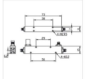
RF Solution offer a wide selection of Coupler for global customers. CP20-F1573-S-1-4GHz is a Coupler in Frequency Range of  $1.0 \sim 4.0$  GHz. It is made of high quality materials under a high standard, the Insertion Loss Max of this product is 0.5 dB, Nominal Coupling is  $20 \pm 1$  dB and Coupling Sensitivity is  $\pm$  0.7 dB. The component has a good working performance and stability, it is ideal for handling a Rated Power of 50 W.
