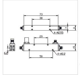
RF Solution offer a wide selection of Coupler for global customers. CP20-F1573-S-1-18GHz is a Coupler in Frequency Range of  $1.0 \sim 18.0$  GHz. It is made of high quality materials under a high standard, the Insertion Loss Max of this product is 0.9 dB, Nominal Coupling is  $20\pm1$  dB and Coupling Sensitivity is  $\pm 1.0$  dB. The component has a good working performance and stability, it is ideal for handling a Rated Power of 50 W.
