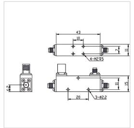
RF Solution offer a wide selection of Coupler for global customers. CP20-F1543-S-2-8GHz is a Coupler in Frequency Range of 2.0~8.0 GHz. It is made of high quality materials under a high standard, the Insertion Loss Max of this product is 0.5dB (Excluding 0.04 dB coupling loss), Nominal Coupling is  $20\pm1$  dB and Coupling Sensitivity is  $\pm$  1.0 dB. The component has a good working performance and stability, it is ideal for handling a Rated Power of 50 W.
