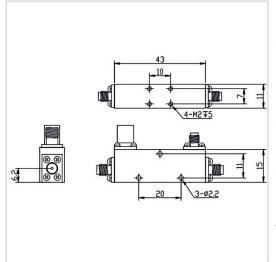
RF Solution offer a wide selection of Coupler for global customers. CP20-F1543-S-2-18GHz is a Coupler in Frequency Range of 2.0-18.0 GHz. It is made of high quality materials under a high standard, the Insertion Loss Max of this product is  $\leq$ 1.2 dB, Nominal Coupling is 20±1 dB and Coupling Sensitivity is ± 1.0 dB. The component has a good working performance and stability, it is ideal for handling a Rated Power of 50 W.
