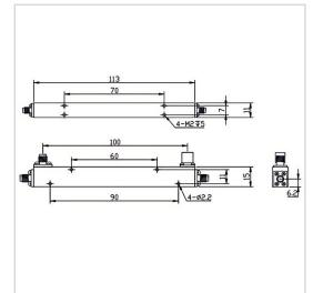
RF Solution offer a wide selection of Coupler for global customers. CP20-F1511-S-0.5-6GHz is a Coupler in Frequency Range of  $0.5 \sim 6.0$  GHz. It is made of high quality materials under a high standard, the Insertion Loss Max of this product is 0.7 dB, Nominal Coupling is  $20\pm1$  dB and Coupling Sensitivity is  $\pm$  0.8 dB. The component has a good working performance and stability, it is ideal for handling a Rated Power of 50 W.
