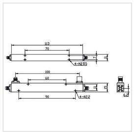
RF Solution offer a wide selection of Coupler for global customers. CP20-F1511-S-0.5-18GHz is a Coupler in Frequency Range of  $0.5\sim18.0$  GHz. It is made of high quality materials under a high standard, the Insertion Loss Max of this product is 1.2 dB, Nominal Coupling is  $20\pm1$  dB and Coupling Sensitivity is  $\pm$  1.0 dB. The component has a good working performance and stability, it is ideal for handling a Rated Power of 50 W.
