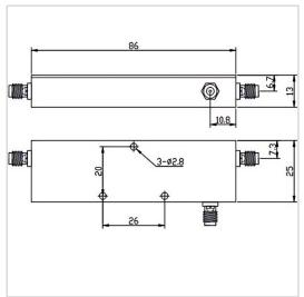
RF Solution offer a wide selection of Coupler for global customers. CP10-F2586-S-0.698-2.2GHz is a Coupler in Frequency Range of  $0.698\sim2.2$  GHz. It is made of high quality materials under a high standard, the Insertion Loss Max of this product is 0.4dB(Excluding 0.45 dB coupling loss), Nominal Coupling is  $10\pm1$  dB and Coupling Sensitivity Max is  $\pm$  0.5 dB. The component has a good working performance and stability, it is ideal for handling a Rated Power of 50 W.
