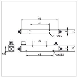
RF Solution offer a wide selection of Coupler for global customers. CP10-F1585-S-0.698-2.7GHz is a Coupler in Frequency Range of  $0.698\sim2.7$ GHz. It is made of high quality materials under a high standard, the Insertion Loss Max of this product is 0.5dB(Excluding 0.45 dB coupling loss), Nominal Coupling is  $10\pm1$  dB and Coupling Sensitivity Max is  $\pm$  1.0 dB. The component has a good working performance and stability, it is ideal for handling a Rated Power of 50 W.
