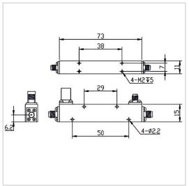
RF Solution offer a wide selection of Coupler for global customers. CP10-F1573-S-1-4GHz is a Coupler in Frequency Range of  $1.0{\sim}4.0$  GHz. It is made of high quality materials under a high standard, the Insertion Loss Max of this product is 0.5dB(Excluding 0.45 dB coupling loss), Nominal Coupling is  $10\pm1 dB$  and Coupling Sensitivity Max is  $\pm$  0.7 dB. The component has a good working performance and stability, it is ideal for handling a Rated Power of 50 W.
