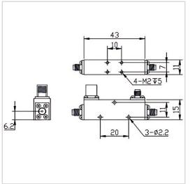
RF Solution offer a wide selection of Coupler for global customers. CP10-F1543-S-2-18GHz is a Coupler in Frequency Range of  $2.0 \sim 18.0$  GHz. It is made of high quality materials under a high standard, the Insertion Loss Max of this product is 0.7dB (Excluding 0.45 dB coupling loss), Nominal Coupling is  $10\pm1$  dB and Coupling Sensitivity Max is  $\pm1.0$  dB. The component has a good working performance and stability, it is ideal for handling a Rated Power of 20 W.
