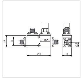
RF Solution offer a wide selection of Coupler for global customers. CP10-F1528-G-6-40GHz is a Coupler in Frequency Range of  $6.0 \sim 40.0$  GHz. It is made of high quality materials under a high standard, the Insertion Loss Max of this product is 1.2dB (Excluding 0.45 dB coupling loss), Nominal Coupling is  $10\pm1$  dB and Coupling Sensitivity is  $\pm$  1.0 dB. The component has a good working performance and stability, it is ideal for handling a Rated Power of 20 W.
