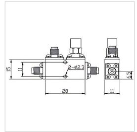
RF Solution offer a wide selection of Coupler for global customers. CP10-F1528-G-27-32GHz is a Coupler in Frequency Range of 27.0~32.0 GHz. It is made of high quality materials under a high standard, the Insertion Loss Max of this product is 1.0dB (Excluding 0.45 dB coupling loss), Nominal Coupling is  $10\pm1$  dB and Coupling Sensitivity is  $\pm$  1.0 dB. The component has a good working performance and stability, it is ideal for handling a Rated Power of 20 W.
