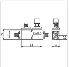
RF Solution offer a wide selection of Coupler for global customers. CP10-F1528-G-18-40GHz is a Coupler in Frequency Range of 18.0~40.0 GHz. It is made of high quality materials under a high standard, the Insertion Loss Max of this product is 1.2dB (Excluding 0.45 dB coupling loss), Nominal Coupling is 10±1 dB and Coupling Sensitivity is ± 1.0 dB. The component has a good working performance and stability, it is ideal for handling a Rated Power of 20 W.
