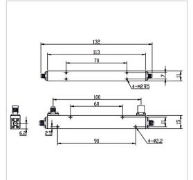
RF Solution offer a wide selection of Coupler for global customers. CP10-F1511-S-0.5-8GHz is a Coupler in Frequency Range of  $0.5 \sim 8.0$  GHz. It is made of high quality materials under a high standard, the Insertion Loss Max of this product is  $\pm 0.7$ dB(Excluding 0.45 dB coupling loss), Nominal Coupling is  $10\pm1$  dB and Coupling Sensitivity Max is  $\pm$  0.7 dB. The component has a good working performance and stability, it is ideal for handling a Rated Power of 50 W.
