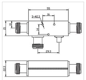
RF Solution offer a wide selection of Coupler for global customers. CP06-F2155-N-2-6GHz is a Coupler in Frequency Range of  $2.0 \sim 6.0$  GHz. It is made of high quality materials under a high standard, the Insertion Loss Max of this product is 1.5 dB, Nominal Coupling is  $6\pm1$  dB and Coupling Sensitivity is /. The component has a good working performance and stability, it is ideal for handling a Rated Power of 30 W.
