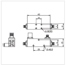
RF Solution offer a wide selection of Coupler for global customers. CP06-F1543-S-2-8GHz is a Coupler in Frequency Range of  $2.0{\sim}8.0$  GHz. It is made of high quality materials under a high standard, the Insertion Loss Max of this product is 0.5 dB (Excluding 1.26dB coupling loss), Nominal Coupling is  $6{\pm}1$  dB and Coupling Sensitivity Max is  $\pm0.7$  dB. The component has a good working performance and stability, it is ideal for handling a Rated Power of 50 W.
