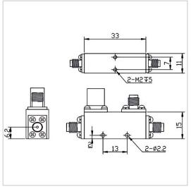
RF Solution offer a wide selection of Coupler for global customers. CP06-F1533-S-6-18GHz is a Coupler in Frequency Range of  $6.0 \sim 18.0$  GHz. It is made of high quality materials under a high standard, the Insertion Loss Max of this product is 0.8 dB , Nominal Coupling is  $6\pm 1$  dB and Coupling Sensitivity Max is  $\pm 0.8$  dB. The component has a good working performance and stability, it is ideal for handling a Rated Power of 50 W.
