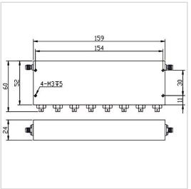
RF Solution offer a wide selection of Band Stop Filter for global customers. BSF-935M960A-S is a Band Stop Filter in Rejection Band of 935~960 MHz. It is made of high quality materials under a high standard, the Pass Band of this product is DC~925MHz / 970~1600MHz, Insertion Loss Max is 2.0 dB and Rejection Min is 40 dB. The component has a good working performance and stability, it is ideal for handling a Rated Power of 20 W.
