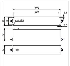
RF Solution offer a wide selection of Band Stop Filter for global customers. BSF-921M960A-S is a Band Stop Filter in Rejection Band of 921~960 MHz. It is made of high quality materials under a high standard, the Pass Band of this product is DC~911MHz / 970~1800MHz, Insertion Loss Max is 2.0 dB and Rejection Min is 40 dB. The component has a good working performance and stability, it is ideal for handling a Rated Power of 20 W.
