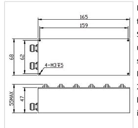
RF Solution offer a wide selection of Band Stop Filter for global customers. BSF-902M928A-N is a Band Stop Filter in Rejection Band of 902~928 MHz. It is made of high quality materials under a high standard, the Pass Band of this product is DC~896MHz / 934~2500MHz, Insertion Loss Max is 2.0 dB and Rejection Min is 45 dB. The component has a good working performance and stability, it is ideal for handling a Rated Power of 20 W.
