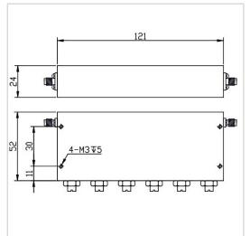
RF Solution offer a wide selection of Band Stop Filter for global customers. BSF-869M894A-S is a Band Stop Filter in Rejection Band of 869~894 MHz. It is made of high quality materials under a high standard, the Pass Band of this product is DC~854MHz / 909~2000MHz, Insertion Loss Max is 1.5 dB and Rejection Min is 40 dB. The component has a good working performance and stability, it is ideal for handling a Rated Power of 20 W.
