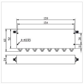
RF Solution offer a wide selection of Band Stop Filter for global customers. BSF-814M849A-S is a Band Stop Filter in Rejection Band of 814~849 MHz. It is made of high quality materials under a high standard, the Pass Band of this product is DC~799MHz / 864~2000MHz, Insertion Loss Max is 1.5 dB and Rejection Min is 45 dB. The component has a good working performance and stability, it is ideal for handling a Rated Power of 20 W.
