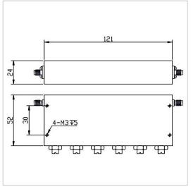
RF Solution offer a wide selection of Band Stop Filter for global customers. BSF-777M787A-S is a Band Stop Filter in Rejection Band of 777~787 MHz. It is made of high quality materials under a high standard, the Pass Band of this product is DC~762MHz / 802~2000MHz, Insertion Loss Max is 2.0 dB and Rejection Min is 45 dB. The component has a good working performance and stability, it is ideal for handling a Rated Power of 20 W.
