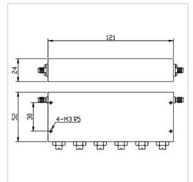
RF Solution offer a wide selection of Band Stop Filter for global customers. BSF-758M803A-S is a Band Stop Filter in Rejection Band of 758~803 MHz. It is made of high quality materials under a high standard, the Pass Band of this product is DC~743MHz / 818~1800MHz, Insertion Loss Max is 2.0 dB and Rejection Min is 40 dB. The component has a good working performance and stability, it is ideal for handling a Rated Power of 10 W.
