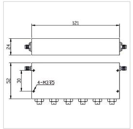
RF Solution offer a wide selection of Band Stop Filter for global customers. BSF-746M756A-S is a Band Stop Filter in Rejection Band of 746~756 MHz. It is made of high quality materials under a high standard, the Pass Band of this product is DC~731MHz / 771~2000MHz, Insertion Loss Max is 2.0 dB and Rejection Min is 40 dB. The component has a good working performance and stability, it is ideal for handling a Rated Power of 20 W.
