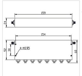
RF Solution offer a wide selection of Band Stop Filter for global customers. BSF-703M748A-S is a Band Stop Filter in Rejection Band of 703~748 MHz. It is made of high quality materials under a high standard, the Pass Band of this product is DC~688MHz / 763~1800MHz, Insertion Loss Max is 2.0 dB and Rejection Min is 60 dB. The component has a good working performance and stability, it is ideal for handling a Rated Power of 20 W.
