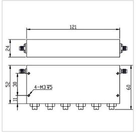
RF Solution offer a wide selection of Band Stop Filter for global customers. BSF-699M716A-S is a Band Stop Filter in Rejection Band of 699~716 MHz. It is made of high quality materials under a high standard, the Pass Band of this product is DC~684MHz / 729~2000MHz, Insertion Loss Max is 2.0 dB and Rejection Min is 40 dB. The component has a good working performance and stability, it is ideal for handling a Rated Power of 20 W.
