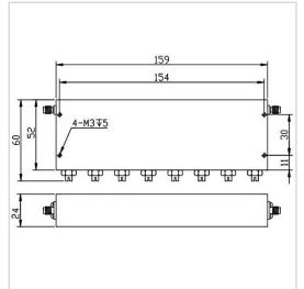
RF Solution offer a wide selection of Band Stop Filter for global customers. BSF-663M698A-S is a Band Stop Filter in Rejection Band of 663~698 MHz. It is made of high quality materials under a high standard, the Pass Band of this product is DC~651MHz / 710~2000MHz, Insertion Loss Max is 2.0 dB and Rejection Min is 50 dB. The component has a good working performance and stability, it is ideal for handling a Rated Power of 20 W.
