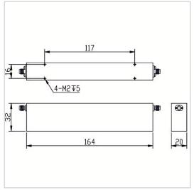
RF Solution offer a wide selection of Band Stop Filter for global customers. BSF-5250M5350A-S is a Band Stop Filter in Rejection Band of 5250~5350 MHz. It is made of high quality materials under a high standard, the Pass Band of this product is DC~5225MHz / 5375~8000MHz, Insertion Loss Max is 3.0 dB and Rejection Min is 80 dB. The component has a good working performance and stability, it is ideal for handling a Rated Power of 10 W.
