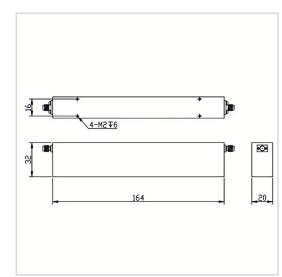
RF Solution offer a wide selection of Band Stop Filter for global customers. BSF-5150M5925A-S is a Band Stop Filter in Rejection Band of 5150~5925 MHz. It is made of high quality materials under a high standard, the Pass Band of this product is DC~5000MHz / 6125~8000MHz, Insertion Loss Max is 2.0 dB and Rejection Min is 50 dB. The component has a good working performance and stability, it is ideal for handling a Rated Power of 10 W.
