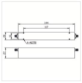
RF Solution offer a wide selection of Band Stop Filter for global customers. BSF-5150M5850A-S is a Band Stop Filter in Rejection Band of 5150~5850 MHz. It is made of high quality materials under a high standard, the Pass Band of this product is DC~5000MHz / 6000~18000MHz, Insertion Loss Max is 3.0 dB and Rejection Min is 50 dB. The component has a good working performance and stability, it is ideal for handling a Rated Power of 10 W.
