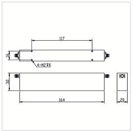
RF Solution offer a wide selection of Band Stop Filter for global customers. BSF-5150M5250A-S is a Band Stop Filter in Rejection Band of 5150~5250 MHz. It is made of high quality materials under a high standard, the Pass Band of this product is DC~5152MHz / 5275~8000MHz, Insertion Loss Max is 3.0 dB and Rejection Min is 80 dB. The component has a good working performance and stability, it is ideal for handling a Rated Power of 10 W.
