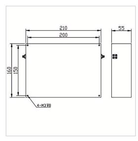
RF Solution offer a wide selection of Band Stop Filter for global customers. BSF-400M600A-S is a Band Stop Filter in Rejection Band of 400~600 MHz. It is made of high quality materials under a high standard, the Pass Band of this product is DC~390MHz / 480~1500MHz, Insertion Loss Max is 2.0 dB and Rejection Min is 60dB@DC-800MHz. The component has a good working performance and stability, it is ideal for handling a Rated Power of 100 W.
